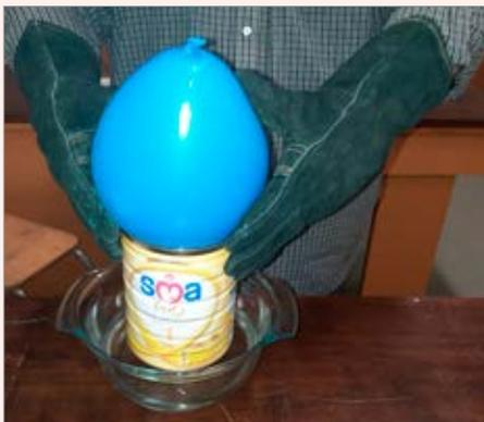
7. After ~2 minutes the whole apparatus can be lifted at the balloon knot. The balloon can also be bounced up and down without the tin slipping off the balloon. For students: "Thinking about your answers to previous questions, can you explain why the balloon and tin do not separate, even when I bounce them up and down vigorously?"
