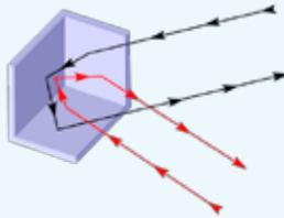
2. If the light is reflected from all three surfaces then it is inverted and rotated. Your own reflection in the three mirrors of a corner reflector will appear upside down and reversed left-to-right. (This is quite different from the reflection in just two mirrors.)
