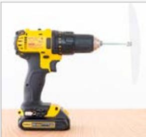
3. Insert the free end of the bolt into the drill and tighten the chuck to hold it in place.
