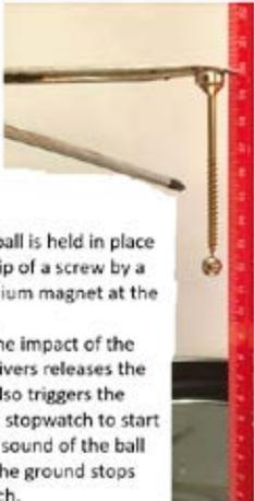
A steel ball is held in place at the tip of a screw by a neodymium magnet at the top. When the impact of the screwdrivers releases the ball, it also triggers the acoustic stopwatch to start and the sound of the ball hitting the ground stops the watch.
