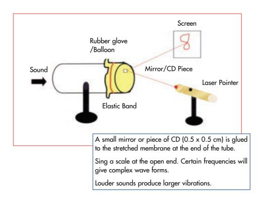
**SAFETY NOTE:** Remind students of the danger of looking into a Laser Beam. Use stands to reduce the movement of the tube and laser.
