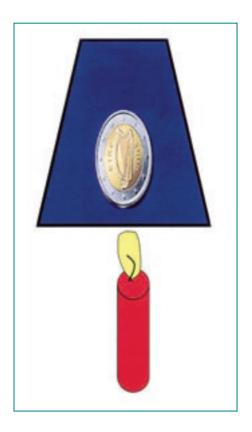
Heat the card directly underneath the coin. The coin conducts the heat away from the card.
