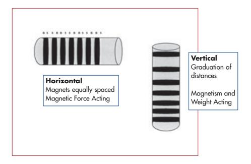
Button Magnets 12.5mm dia (available from Peat's) fit neatly into the test tube.
