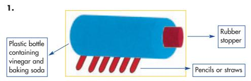
Place a teaspoon full of baking soda and 10mls of vinegar inside the plastic bottle. Quickly replace the rubber stopper. After a few seconds the build up of pressure from the carbon dioxide causes the stopper to fly off in one direction while the bottle shoots back in the opposite direction. By placing the bottle on rollers such as pencils the effect is enhanced.
